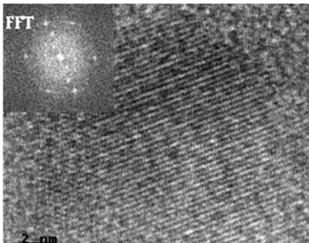
**Fig. 5** The fast Fourier transform (*inset*) and inverse fast Fourier transform of a single Si NP obtained by HRTEM
