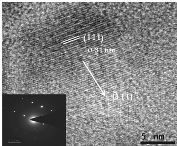
**Fig. 4** HRTEM image of a single Si NP, showing the [111] plane and their corresponding electron diffraction pattern (*inset*)
