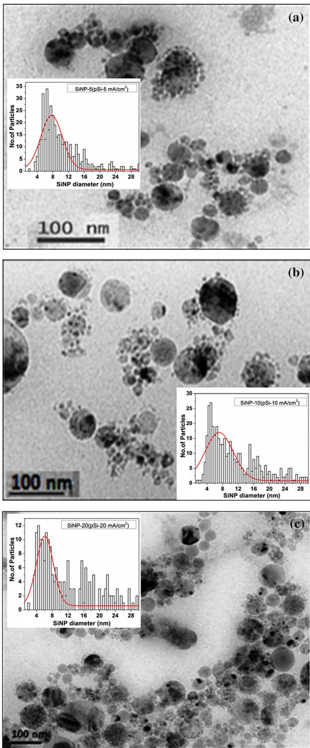
**Fig. 2** TEM images and corresponding histograms (*inset*) of Si NPs obtained by femtosecond laser ablation of pSi targets prepared at different etching current densities. **a** pSi-5 mA/cm<sup>2</sup>, **b** pSi-10 mA/cm<sup>2</sup>, and **c** pSi-20 mA/cm<sup>2</sup> (The *solid lines* in the *insets* represent Gaussian fits of corresponding size distribution)
