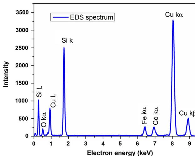
**Fig. 3** Energy dispersive X-ray spectrum of Si NPs
