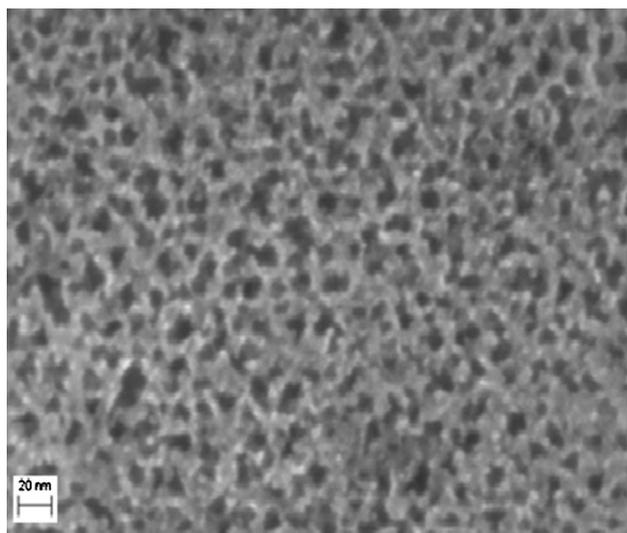
**Fig. 1** FESEM image of nanostructured porous silicon (pSi) prepared at current density  $J = 10$  (mA/cm<sup>2</sup>) by electrochemical etching of Si
