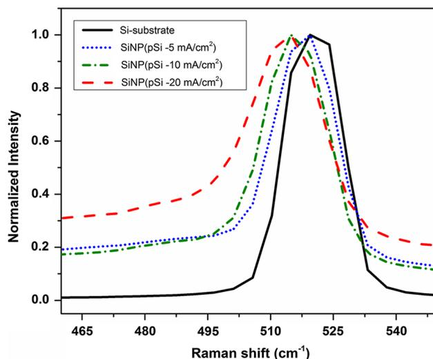
**Fig. 7** Raman spectra of Si NPs synthesized by femtosecond laser ablation of pSi prepared at different etching current densities
