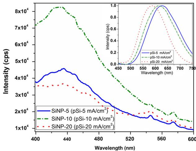
**Fig. 8** Photoluminescence spectra of pSi before ablation (*inset*) and that of the colloidal Si NPs generated by laser ablation of porous silicon prepared at various etching current densities (Note: The concentration of Si NPs is expected to be different in different liquid samples. Hence the changes in intensity may not be interpreted in terms of physical parameters like size, etc.)
