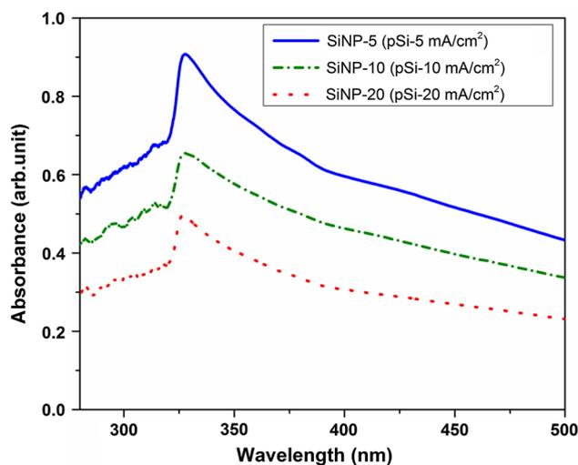
**Fig. 6** UV–Vis absorption spectra of colloidal Si NPs generated with different pSi targets by laser ablation
